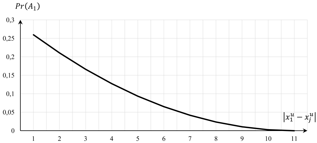
Figure 16. Probability of error in determining the sign of the relative distance, where |x_1^u - x_j^u| – true distance between objects Ob_1^a and Ob_j^a
