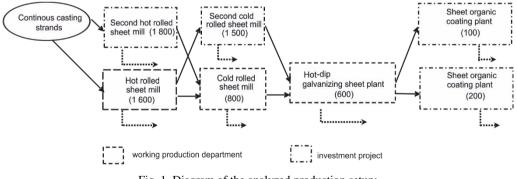
Fig. 1. Diagram of the analyzed production setup; production capacity in thousand tonnes is given in parentheses
